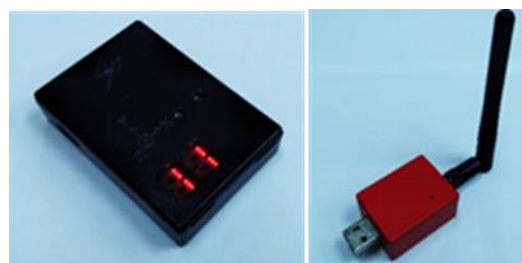
Figure 2. (Left) DSP wireless 9 axis motion sensor (Right) High power data transceiver
