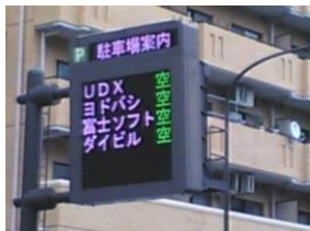
Figure 1 An example of parking guidance Board
