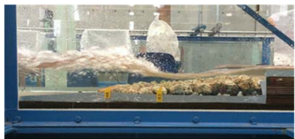
Figure 3. Flow condition for F_1=3 , i=10\% , and h_d/h_1=5.31 .
