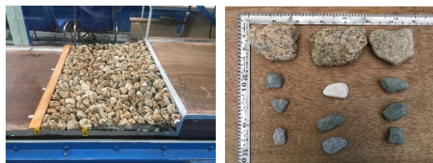
Figure 1. Physical model of stacked boulders in sloping apron below drop.
