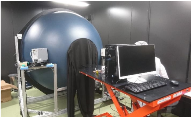
Figure3. Integrating sphere device for flat test.
