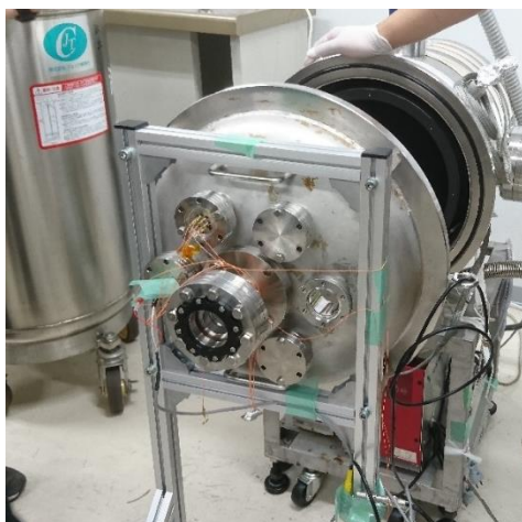
Figure4. Thermal vacuum testing machine.
