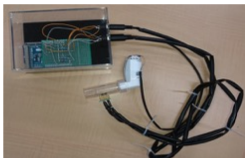
Figure1. Inhaler and measurement system of spray velocity
