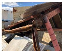
Fig.13 Damaged leg
