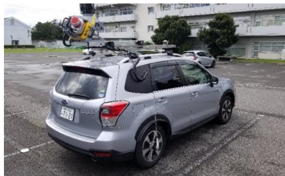
Figure 1. Mobile Mapping System (Trinble MX9)
