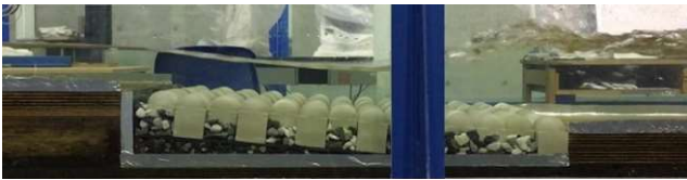
Figure 2. Flow condition for F_1=1, i=1/10 , and h_d/h_1=1.89 .
