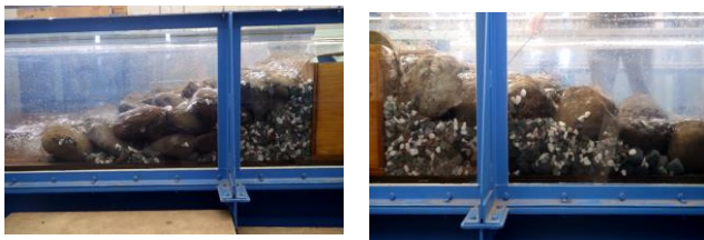
Figure 2. Flow conditions in stacked boulders for i = 1/5 slope, h_c = 3.3 cm, d_{50} = 0.30 m (Right photo: cobble stones, Left photo: flat stones)
