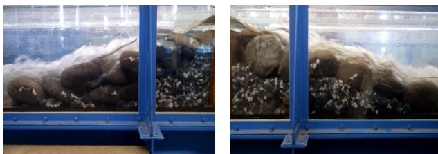
Figure 4. Flow conditions in stacked boulders for i = 1/5 slope, h_c = 6.6 cm, d_{50} = 0.30 m (Right photo: cobble stones, Left photo: flat stones)
