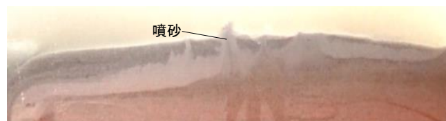
Fig.7 Snapshot of Sand boiling after lateral flow (Case 8)
