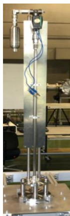
Fig.1 vertical single-stage light gas gun
