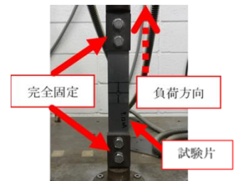
Figure 2. Test specimen attached to fatigue testing
