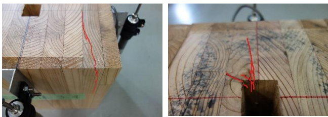
Figure4. Cracks of the specimens
