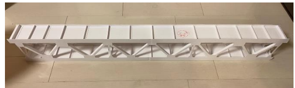
Figure 1. Plate Girder Bridge
