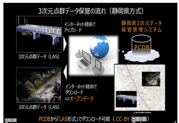
Figure 1. Flow of 3D point cloud data storage [3] (Shizuoka prefecture method)
