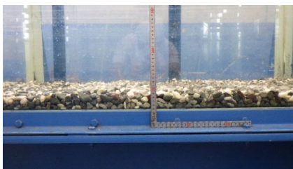
Photo 1 Gravel thickness (about 4 cm) Photo 2 Installation of gravel flatbed Photo 3 Steel mount at downstream end
