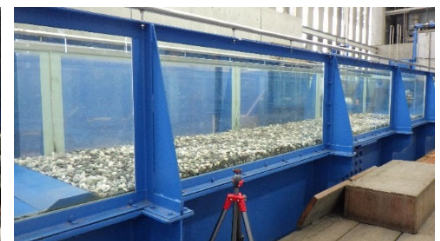
Photo 1 Gravel thickness (about 4 cm) Photo 2 Installation of gravel flatbed Photo 3 Steel mount at downstream end
