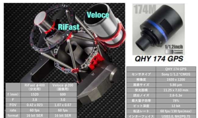
Figure 2, Observation system telescope and camera
