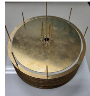
Figure 2. Manufactured fixed capacitor (32nF)
