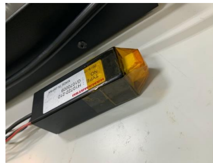
Figure 2. Photograph of the detector constituted with a CsI(Tl) scintillator and a photomultiplier-tube.
