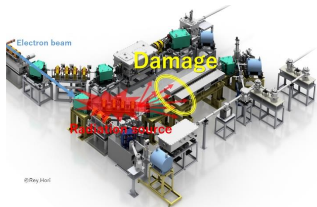
Figure 5: Explanation of the radiation source point affecting the undulator device.
