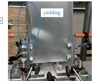
Fig.4 Fracture shape at minimum cross section
