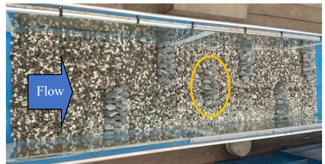
Photo 1. Installation of stacked boulders
