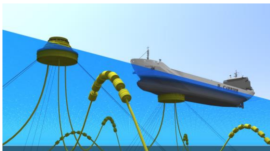
Figure 1 Small float of subsea hydrogen production and storage facility and SLWRs
