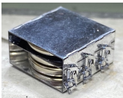
Figure3. Six-legged MEMS micro-robot with built-in button battery.
