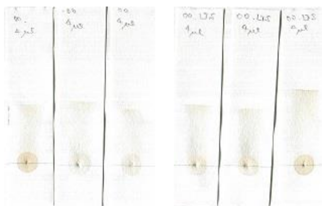
Fig. 2. Result of experience. 3 sheets on the left is no ultrasonic, 3 sheets on the right is irradiated ultrasonic.
