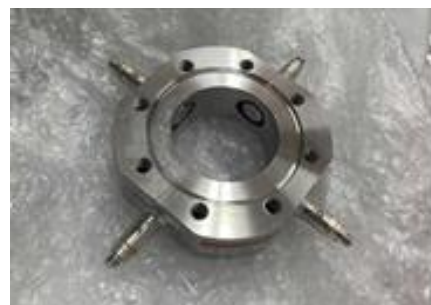
Figure 2. The 4-electrode beam position monitor.
