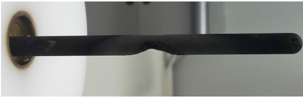
Figure 2. Worn internal electrode
