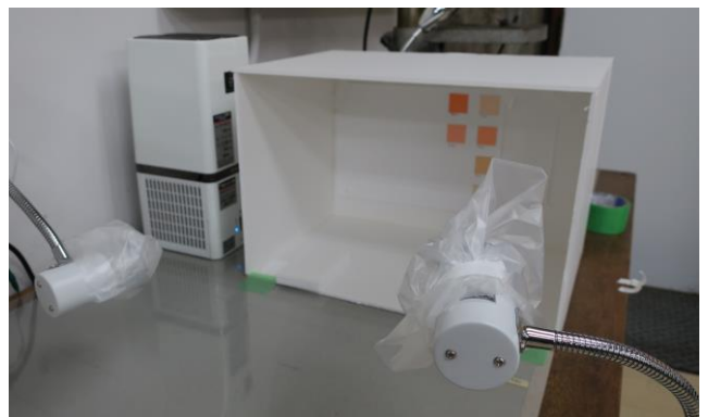
Figure 1. Internal diffusion chamber for spectral reflectance measurements.
