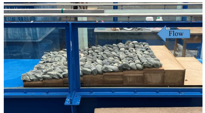
Photo 1 Installation of assembled boulders
