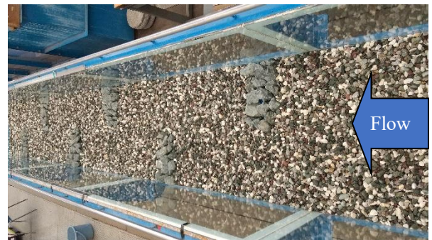
Photo 2. Installation of stacked boulders (Case1)
