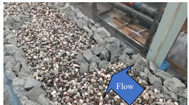
Photo 2. Installation of stacked boulders (Case2)
