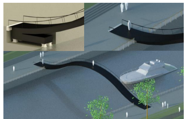
Figure 6. Image of installed the inflected arch bridge
