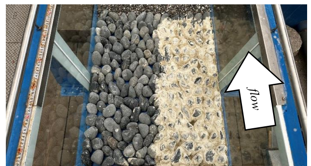
Photo1. Installation of assembled boulders
