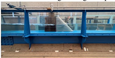
b) Flow condition around trapezoidal elliptical pier
