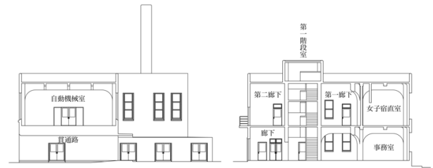
Figure4. cross-sections of Senju telephone office
