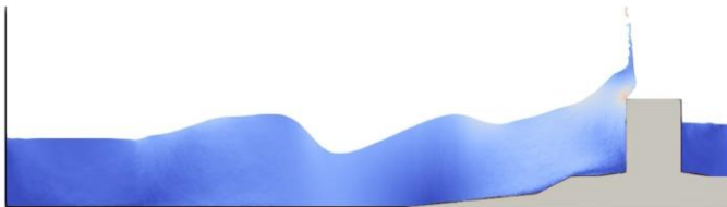
Figure 4 Behavior at maximum wave pressure (Case2)
