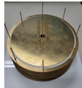
Figure 2. Photo of manufactured slip ring (Multi fin capacitor)
