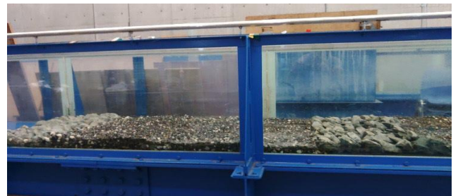
Photo 1. Installation of gravels and assembled boulders
