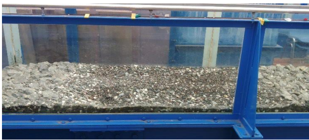
Photo 4. Bed profile after 10 hours.
