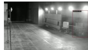
Fig.2 The detection result (The detected smoke)
