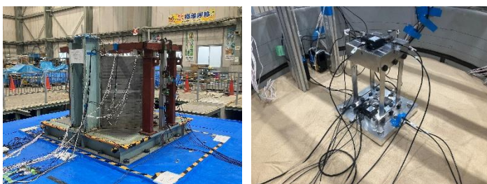
(1) Shear soil tank and Vibration table (2) Ground surface Photo 1. Experimental apparatus
