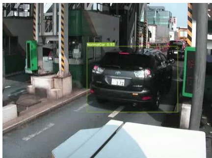
Figure 1. Example of vehicle detection result
