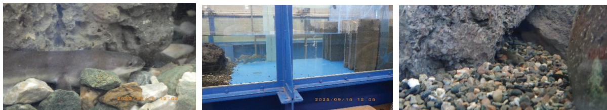
a) Eel inside oxidized slag boulders b) Swimming fishes upstream of boulders c) Amur goby inside oxidized slag
