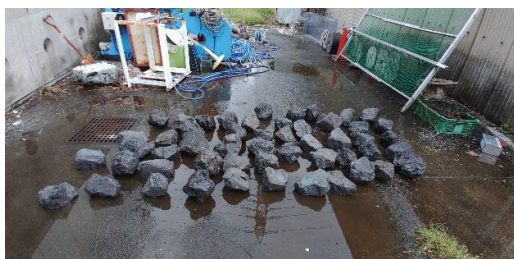
Photo 1 Oxidized Slag Boulders (tested 52 boulders).
