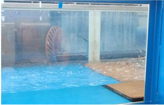
Photo 2 Flow conditions downstream of fish passage (Case1)
