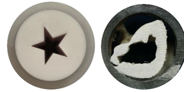
Figure 5. Contracted cross-section after combustion (left: before combustion, right: after combustion)
